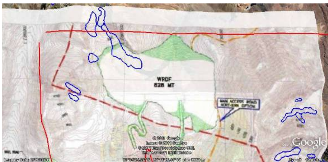
Project map from Minera Andes' EIA compared with glacier inventory shows glaciers in waste facility
