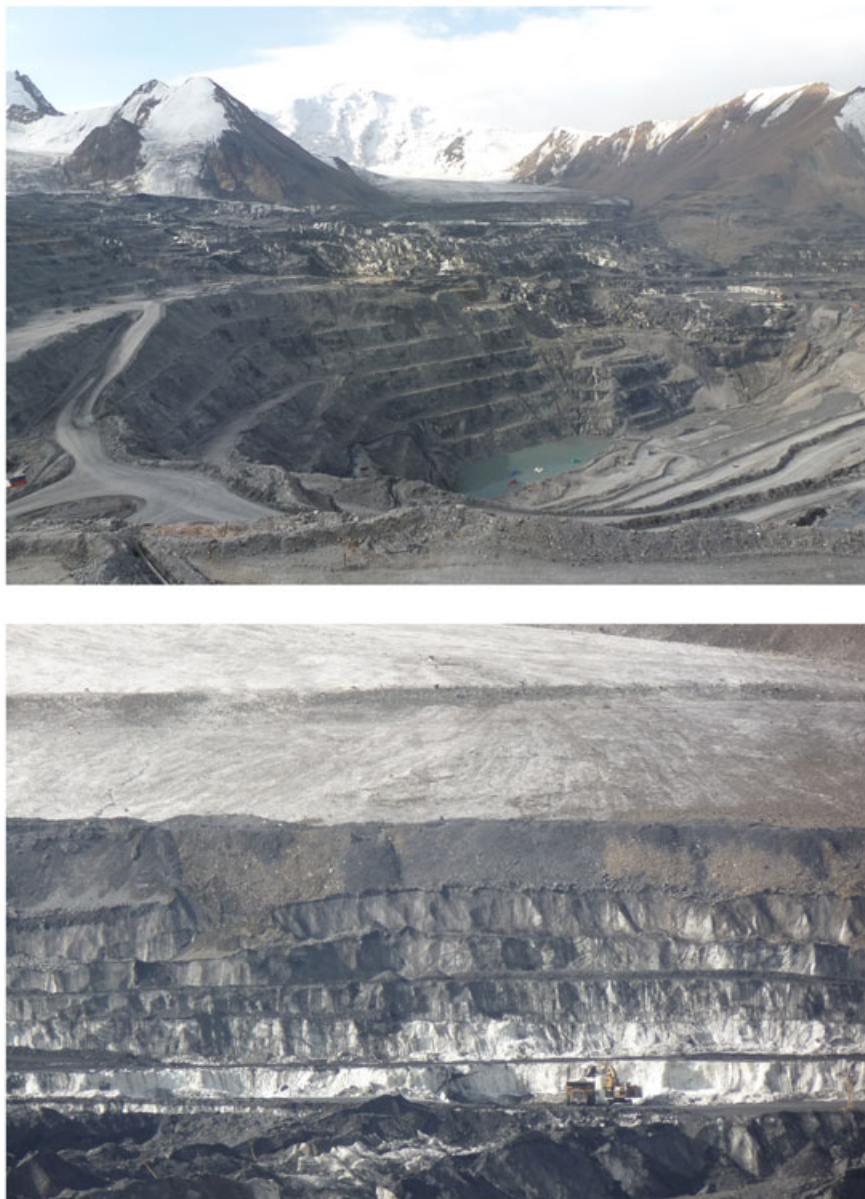
Figure 2. Glacier ice is being excavated at Kumtor mine in Kyrgyzstan (photos by Zbynek Engel)
