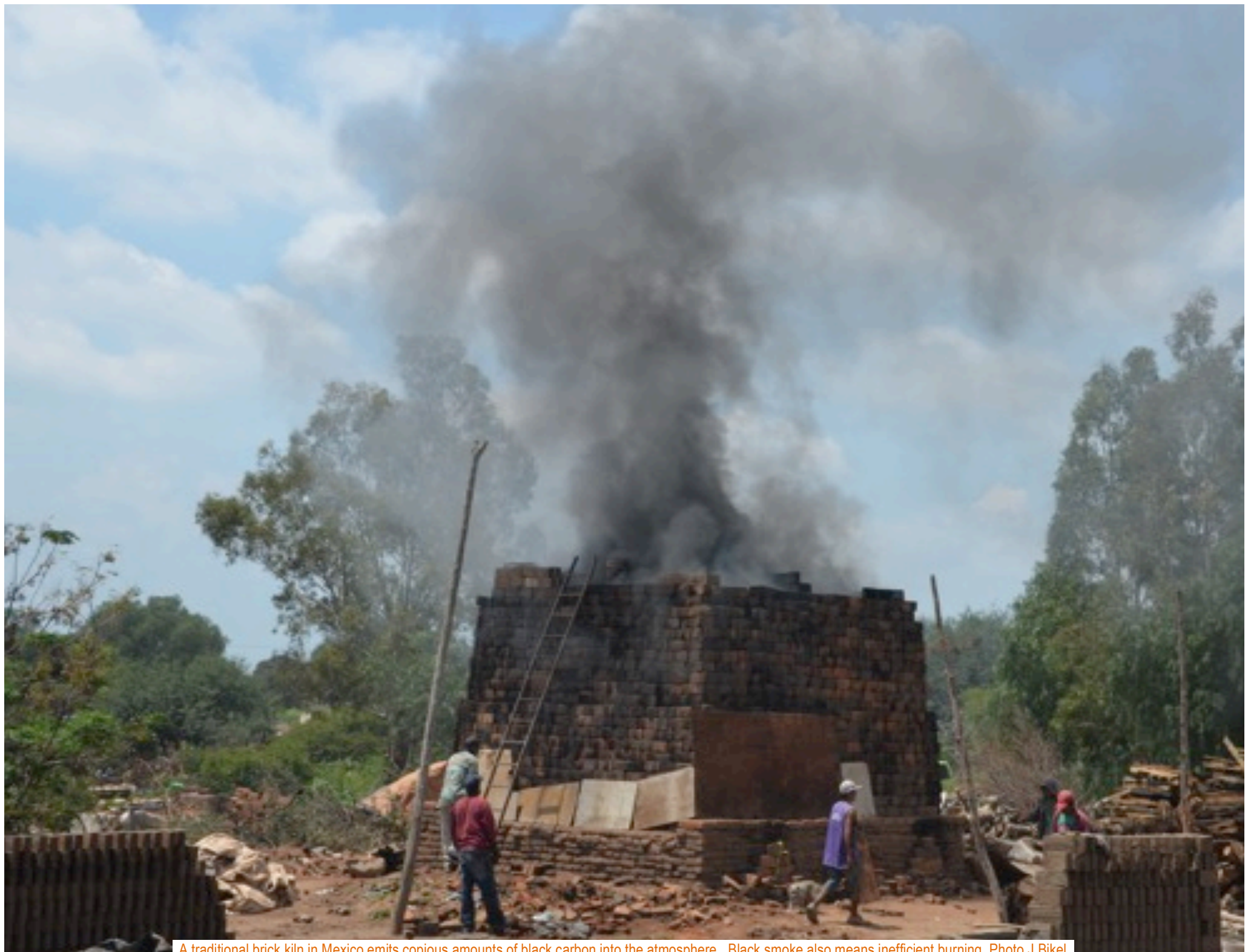
A traditional brick kiln in Mexico emits copious amounts of black carbon into the atmosphere. Black smoke also means inefficient burning. Photo J. Bikel
