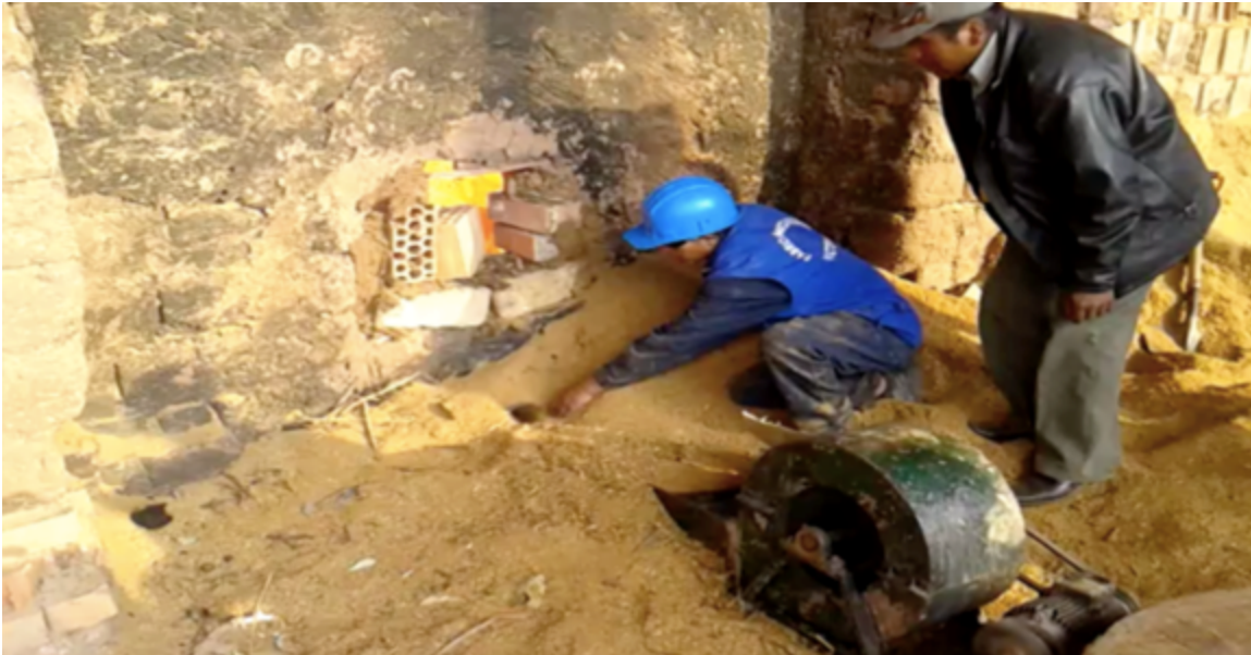
Public officials visit brick production site to witness fuel-efficient blowers installed in traditional brick ovens.
