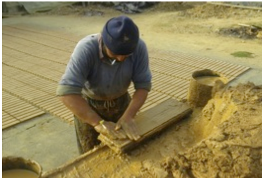
Labor-intensive hand crafted bricks vs mechanical press producing hollow core (uniform and less material used)
