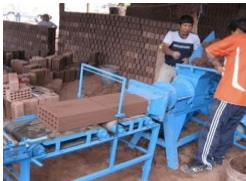
Labor-intensive hand crafted bricks vs mechanical press producing hollow core (uniform and less material used)
