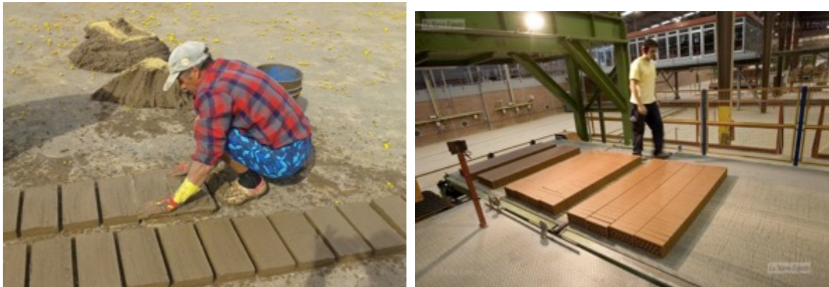
Traditional vs. Modern Technologies used to Set Bricks to Dry; Left: Chile, Right: Spain
