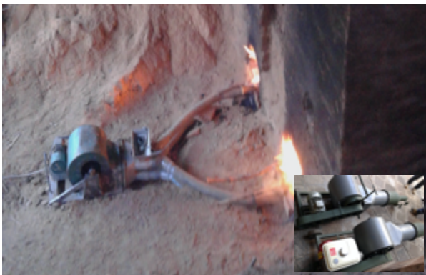
Retrofitting a blower to fuel intake greatly lowers fuel costs and improves burning efficiency
