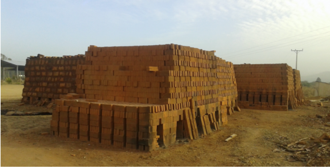
Three traditional brick ovens in Cauquenes Chile. The kiln in the back left has been sealed and is ready for firing.
