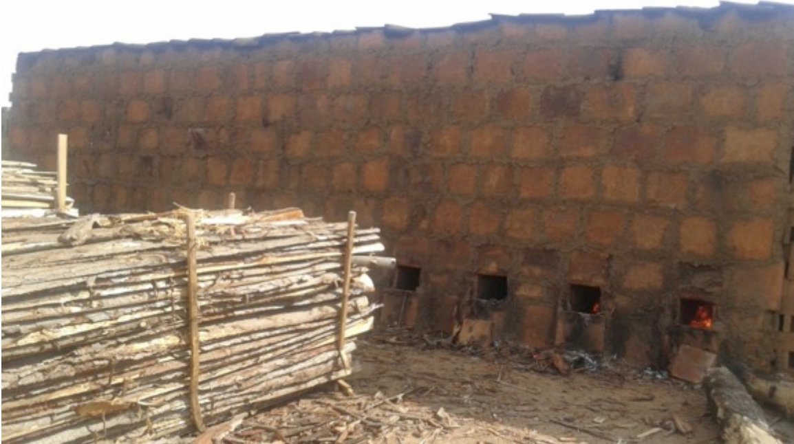
Raw wood fuel, poor kiln design, added to no oxygenation result in improper combustion and unnecessary contamination.
