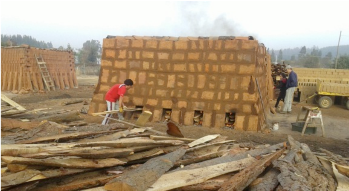
Workshop participants inspect brick kiln oven as it is fed fuel
