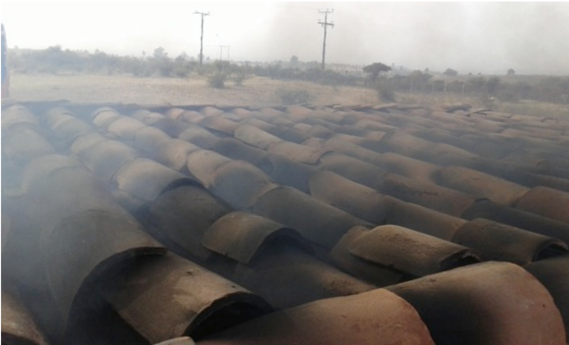
Black Carbon and other emissions result from improper buring techniques.
